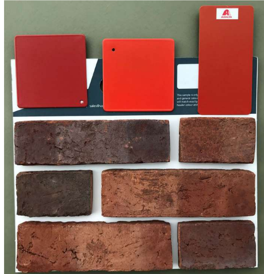
One of several brick types being considered alongside a range of standing seam colours
