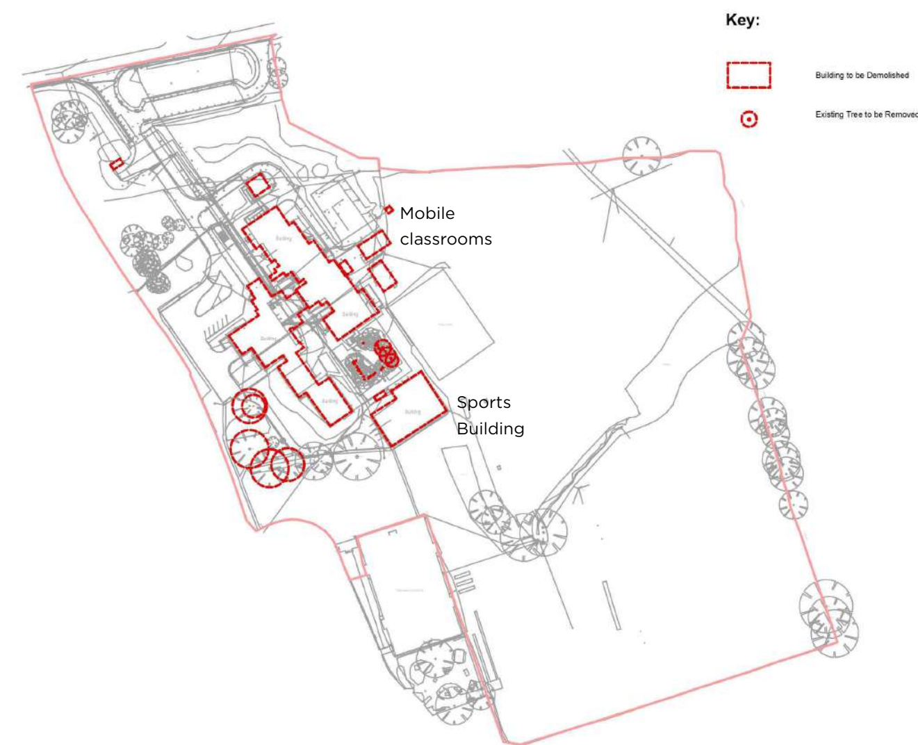
Diagram indicating demolition locations
