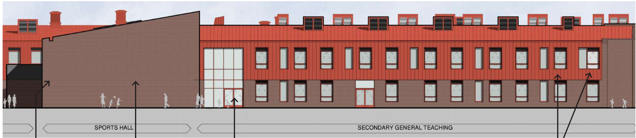
Exposed rainwater downpipes
