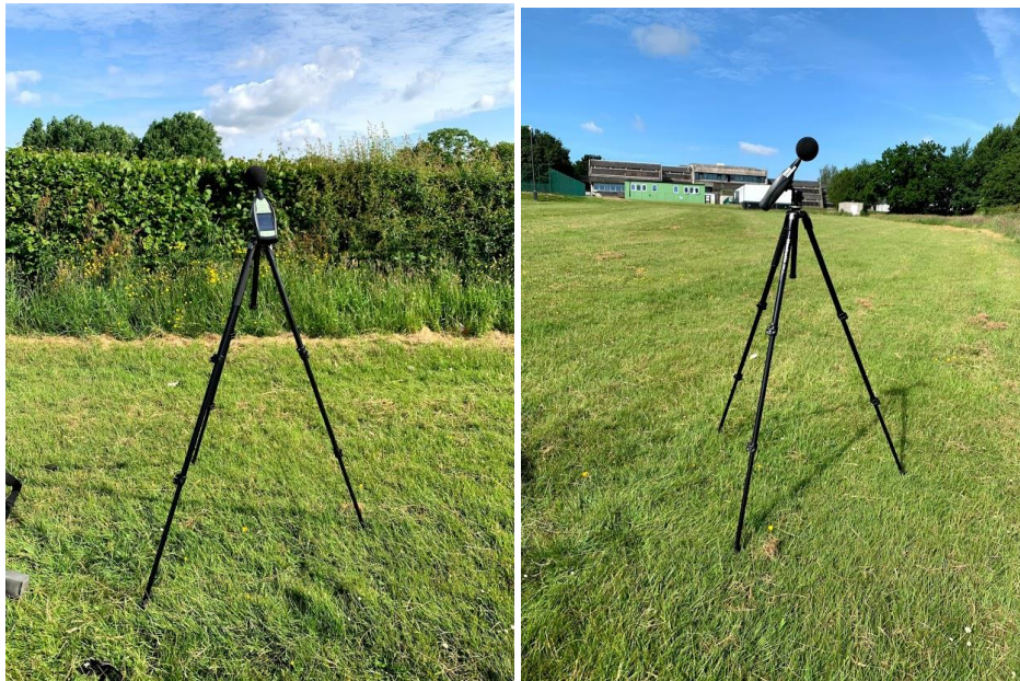
Figure 10: Sound level meter at location 2
