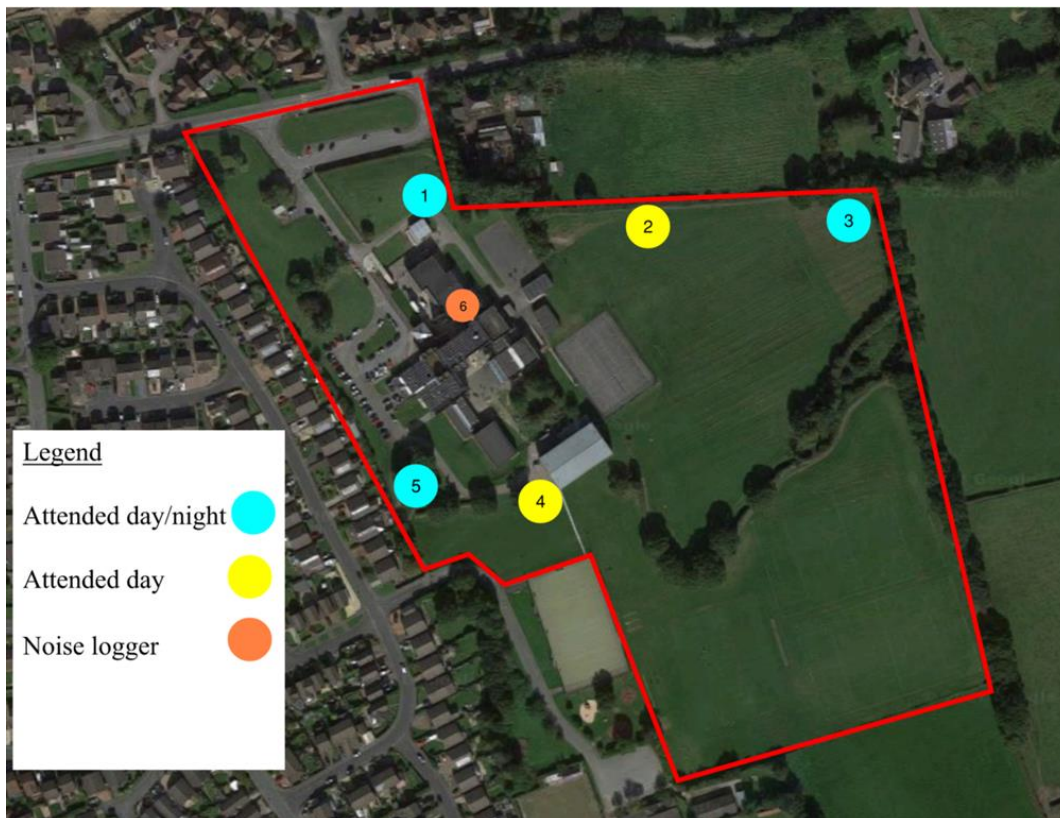
Figure 6: Baseline noise survey measurement locations.
