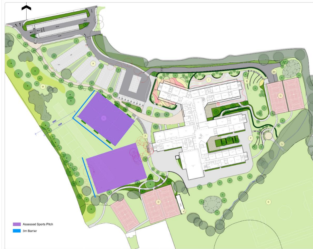
Figure 3: Layout showing noise barriers around the proposed sport pitches.
