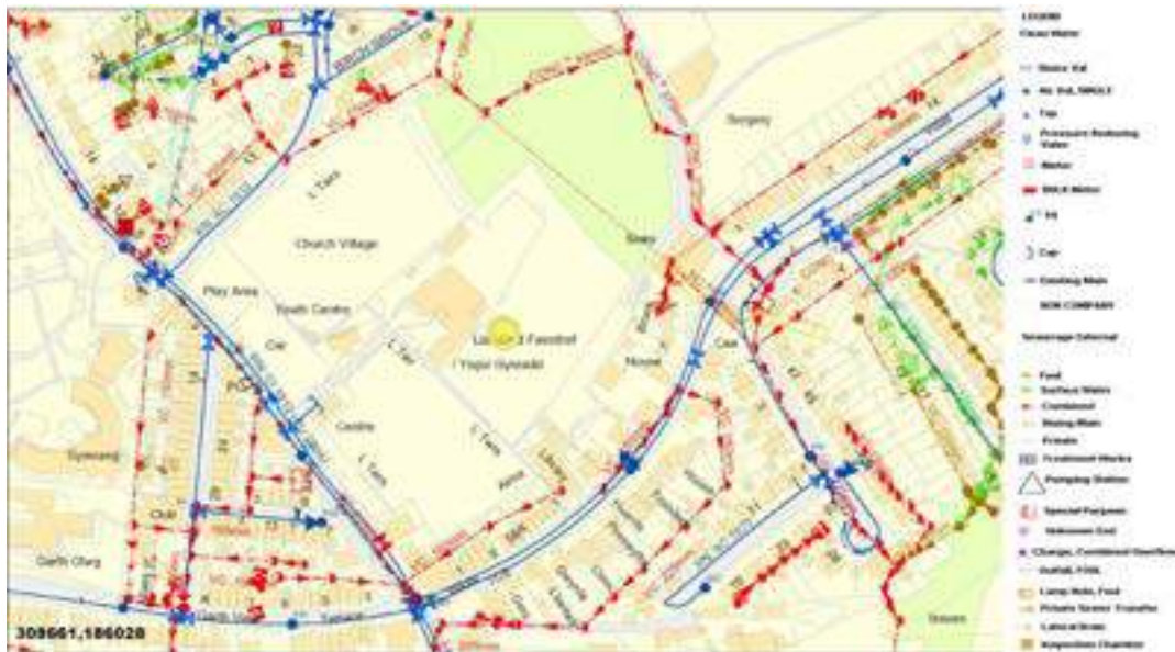
Figure 8: Public sewers plans (DCWW)
