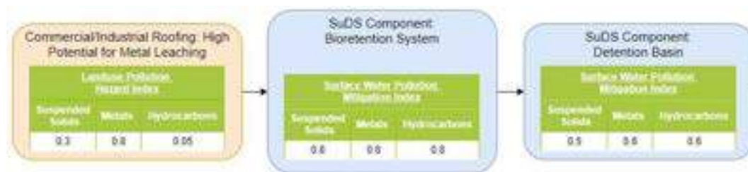
Figure 14: Roof Treatment Train (Simple Index)
