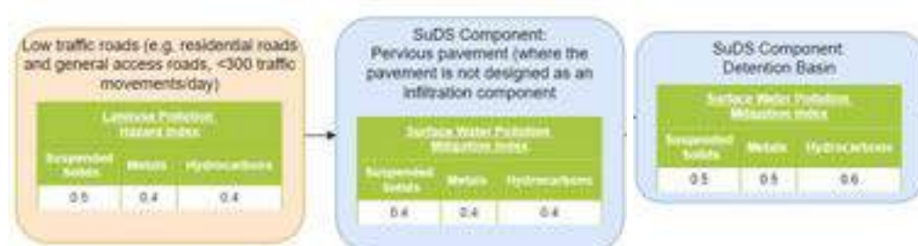
Figure 16: Site Access Road Treatment Train (Simple Index)
