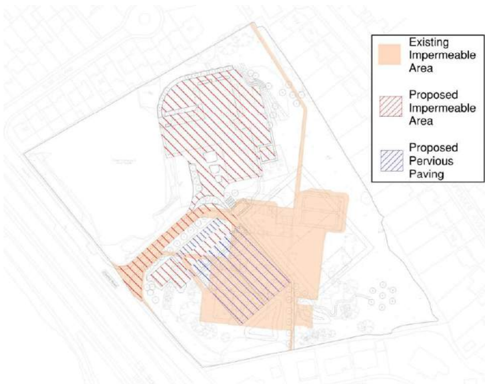
Figure 3: Penygawsi Primary School impermeable area plan
