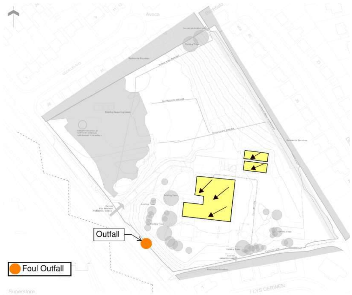
Figure 10. Penygawsi existing foul outfall and catchment
